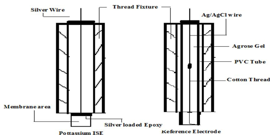
Figure 1: The ISE Modules of potassium and Reference PVC rod
